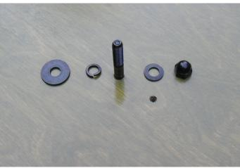
**13.** Attach treadle to wheel with parts 8. Take the plastic cap, lock nut, and washer off large silver assembled bolt. Put the bolt through wheel, front to back. Put washer and lock nut on end of bolt, where it comes out the back of the wheel. Tighten with wrench and flat screwdriver.
