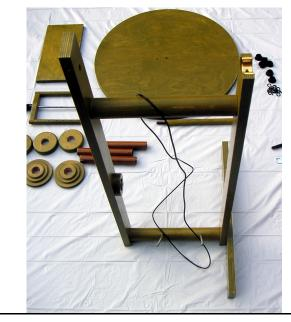
8. Using wooden tapping helper, tap treadle hinges (those bent rods) into holes on the foot rail. Be sure to tap both sides a little at a time, equally, so everything goes in square. When they're in all the way, you'll notice a change in tone when hammering.
