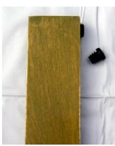
Tap black plastic buffers (shown in #9 and #10 in parts photo) into the holes in bottom of foot rail (#8)
