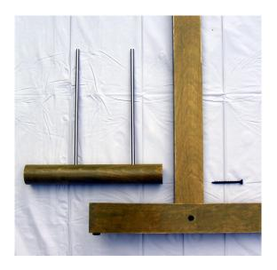
7. Now, build the treadle. Get wooden pieces 5 and 11, the plastic parts and screws (one of the shortest ones and one slightly longer) in 9 (except the buffer that we already used) and bent metal rods (13). Attach the plastic cup to wooden piece 11 (footman) with the shortest screw. Tap the 2 black plastic bushings into the sides of the treadle (5), tapping the short sides of bent rods into bushings. Thread rubber rod into hole in top left of treadle and using longer screw, fix in place.
