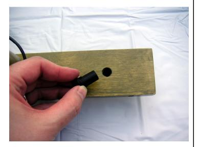
14. Making sure drive band is between wheel and footman, slip plastic ring over plastic cup on treadle footman and place the whole thing over the silver bolt with bearing that you just installed. Move ring down to the edge of the cup to hold in place. The two mouse ears on ring are for removal, should you ever need to.
